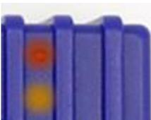
The LCD Sensor has 2 specific status LEDs (yellow and red) which will light up and be blinking if a monitored sensor's status is warning or critical, respectively (see below on the example pictures).
